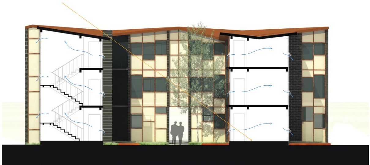
Figure 6. 12 Section: Sunlight and Ventilation
